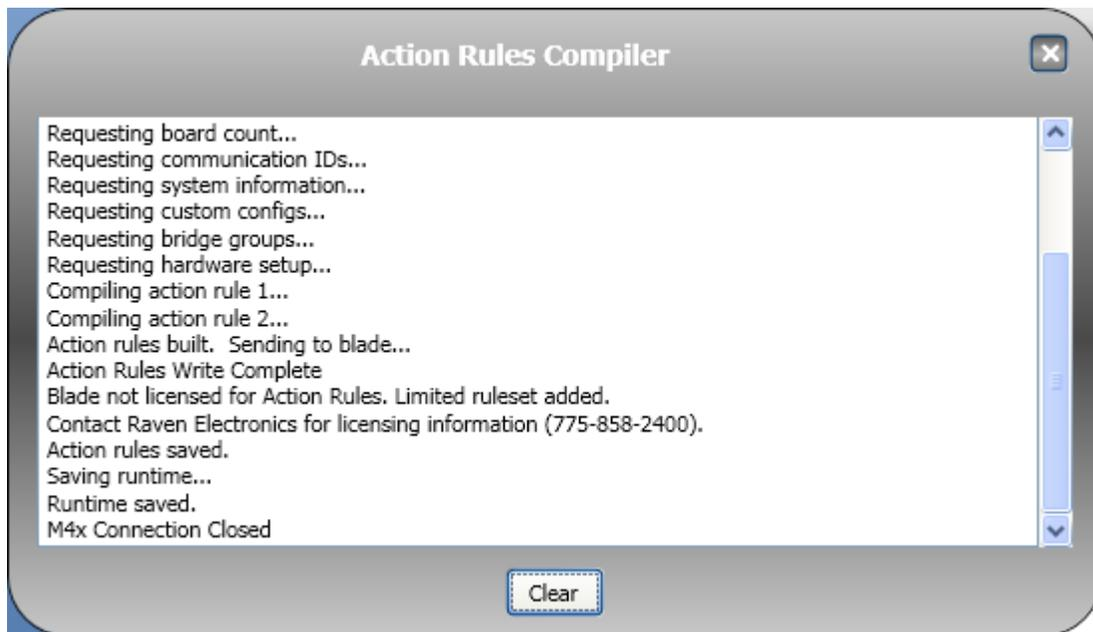
After you select the Write Rules to Blade command, you should see a compiler screen like the one in screen shot above. You should see M4x Connection Closed on the last line of the compiler screen.
