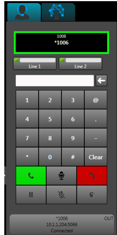
Figure 5-2: The SIP phone control. This dial pad is used to manage SIP and traditional phone line calls.
